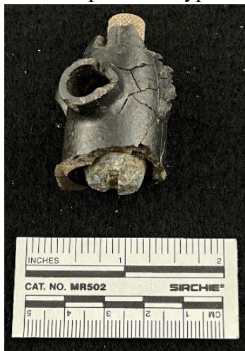
Figure 16: 2021.0403m235. Thermocouple safety valve
